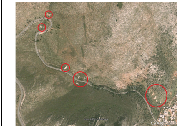
Figure 11. A series of concrete check-dams built uphill of the town of Nea Makri a few months after the 1995 fire of Penteli mountain (Google Earth image 2004)
