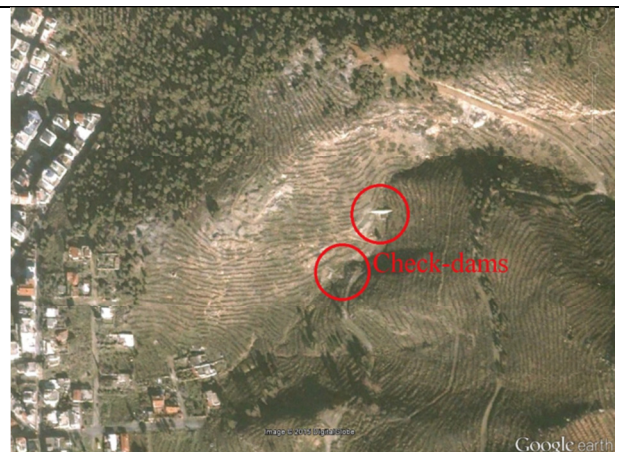
Figure 6. Log-barriers on the slopes along the contours and 2 check-dams, constructed in a ravine after the July 22, 1998 fire on Hymettus mountain, near the suburb of Kareas, Athens, Greece. Kareas is downhill from the burned area. The main restoration objective was soil erosion prevention and flooding protection (Google Earth image, 2001).
